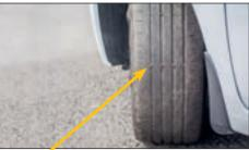
The wear indicators in these major tread grooves are worn down almost to the level of the rest of the tread. This tyre is worn down.
