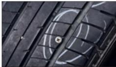
Do not remove a nail or screw embedded in the tyre until you reach a garage. Removal will cause the tyre to deflate rapidly.
