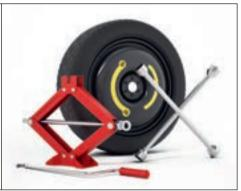
A spare tyre could differ in size from a normal tyre. It is used in emergency situations only. Replace the tyre as soon as possible and drive a maximum of 80 km/h
