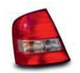
Retro-reflectors come in various colours and ensure that vehicles are visible when stationary in the dark.
